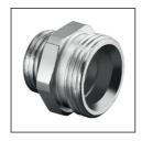
Nipple, nickel plated Port G ½: self sealing Port G ¾: with tapered sealing according to DIN EN 16313 (cone "Euro") G ½ male x G ¾ male Item no. 1028161
