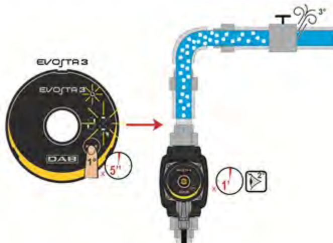
Figure 9: Automatic venting of the pump
