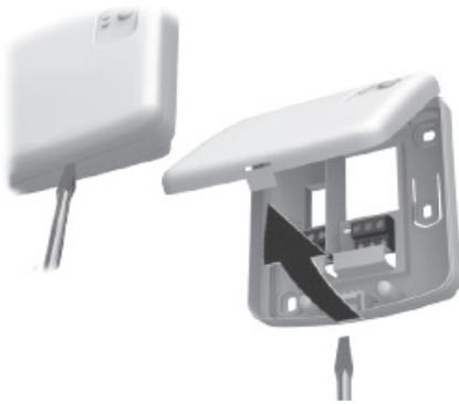
3 Mount the wiring plate to the wall or wallbox.
