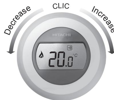
The display changes to current room temperature again after five seconds have passed. Then the thermostat tries to maintain the set temperature as accurately as possible. The setting temperature can be checked by turning the dial one 'click' to the left or right. It will flash up for a few seconds, before returning to the display of room temperature again.
